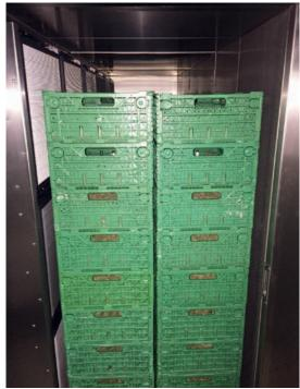
Stacked for drying -Three drying modules accommodate four trolleys with ten trays of cannabis buds each.
