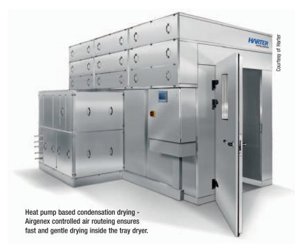
its operating procedure. Harter responded by building a hygienically designed stainless steel tray dryer. Its drying chamber consists of three modules with a floor space the size of a standard European pallet each. The tray dryer was designed to hold the existing harvest trays, as desired by the customer, and is 3,900 mm long, 2,150 mm wide and 2,340 mm high.
